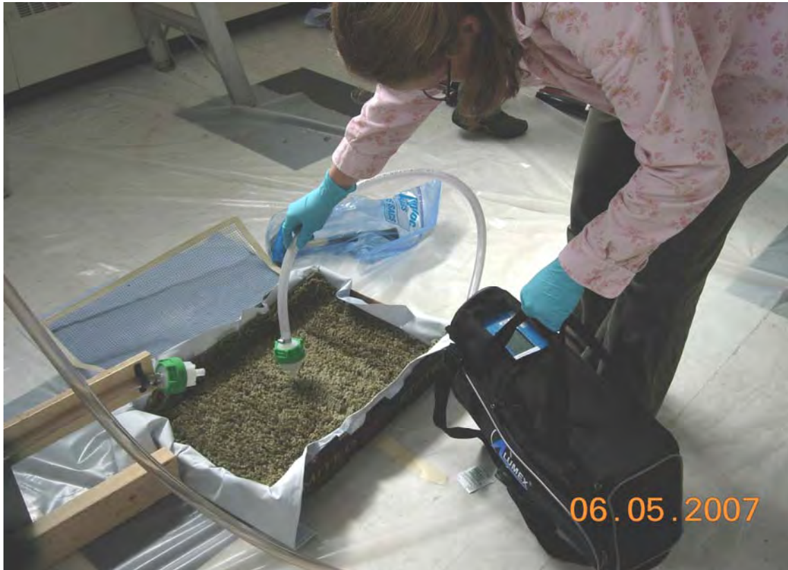
Figure B-3. Taking near-surface mercury measurements.
