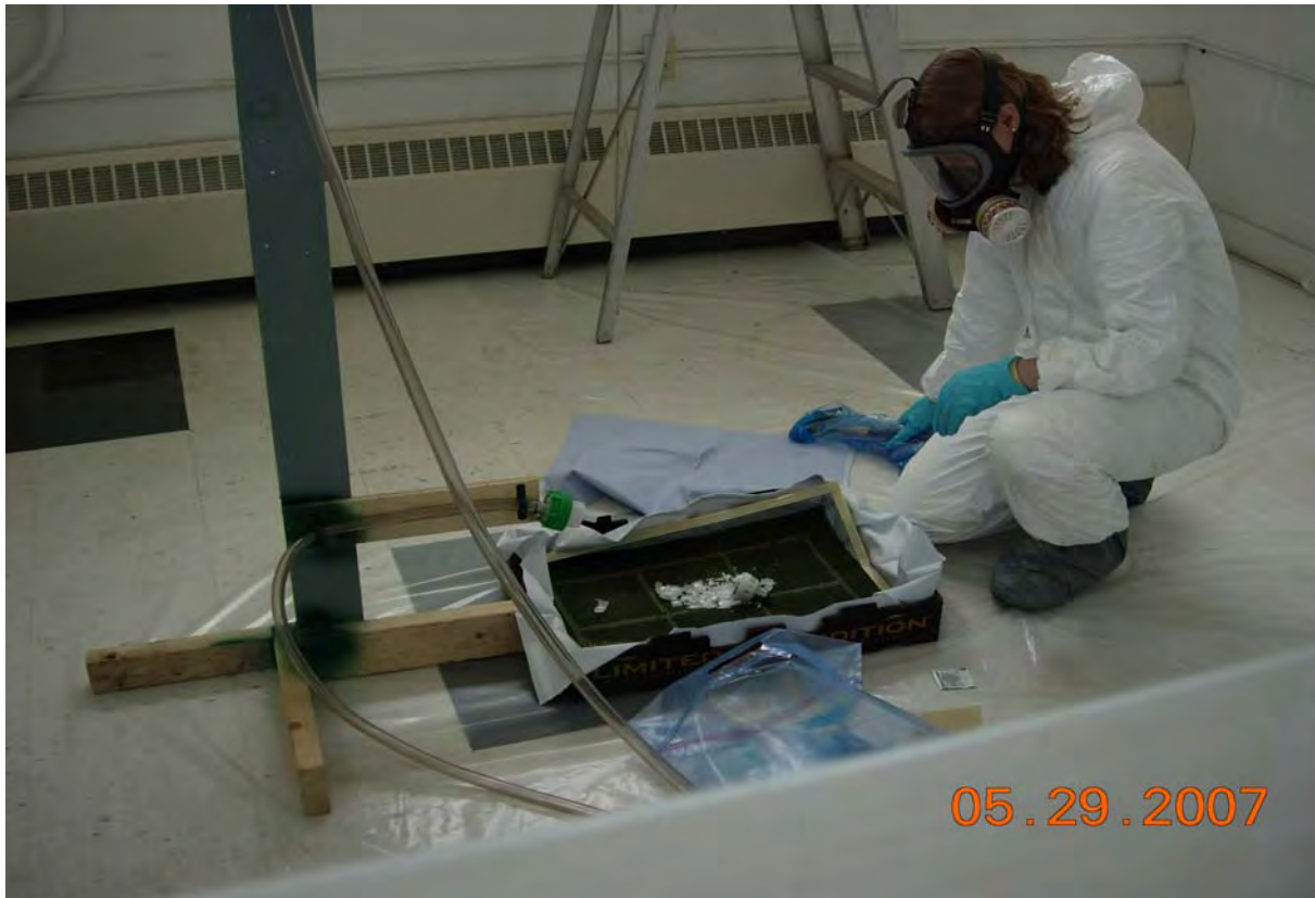
Figure 5-3. Thoroughly broken CFL
