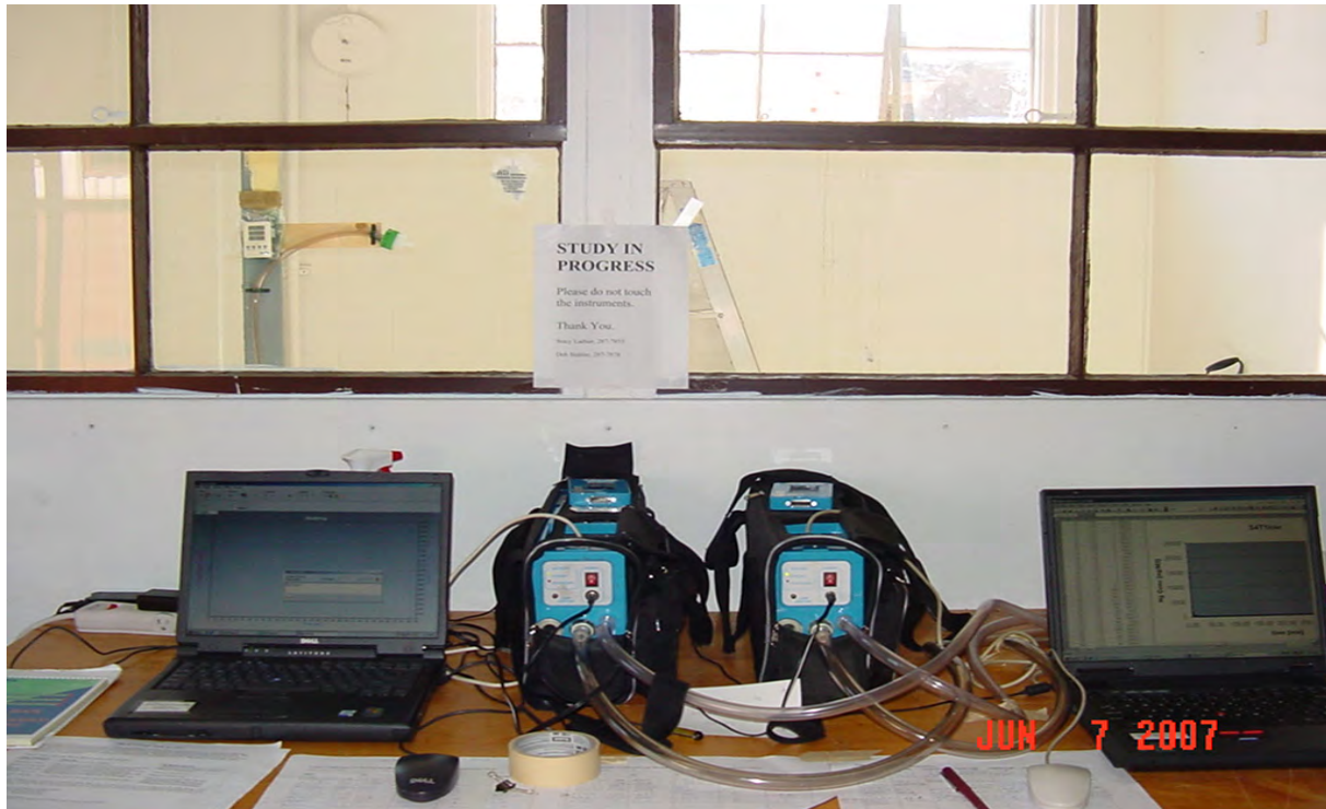
Figure 5-4. Lumex RA 915+ mercury analyzers connected to laptops
