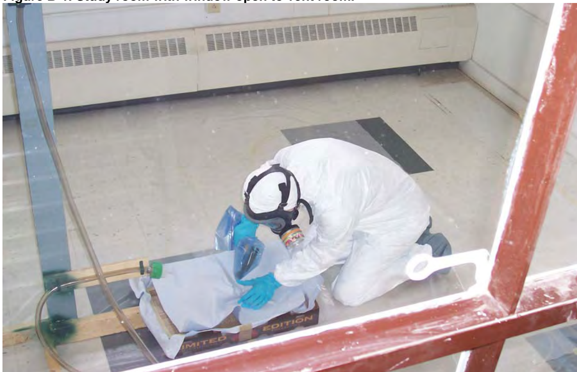
Figure B-2. Breaking a CFL.
