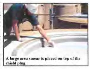
performed on two spent fuel vertical concrete casks. The highest spent fuel cask reading with the Elcometer was 1.1 µg/cm<sup>2</sup>. All salt levels appear to be very low. Additional samples were taken and sent for offsite laboratory analysis.
