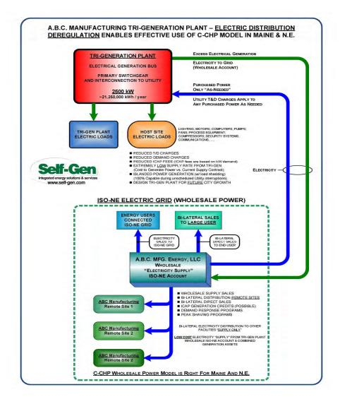
Diagram: C-CHP (Combined Cooling Heat & Power) Facility Electrical Distribution under Deregulated Structure, Source: Self-Gen, Inc
