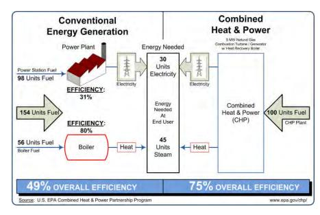
Figure 2-3: Separate Heat and Power Production versus Combined Heat & Power
