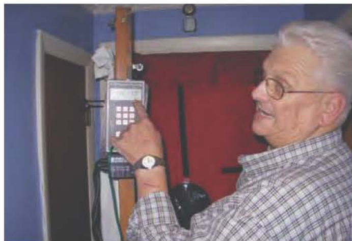
A certified Residential Energy Auditor with York County Community Action is performing a blower door test, which assists in finding air leaks.
