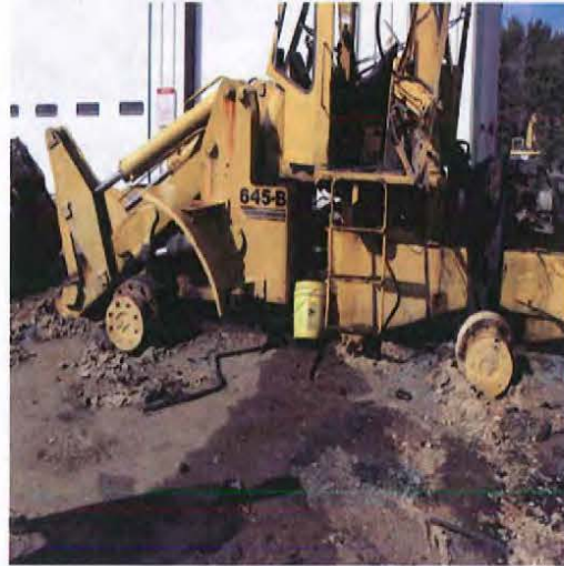
Problem: Vehicle and equipment maintenance with no fluid management controls.
