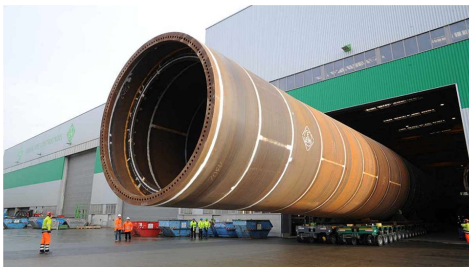
Figure 3-11. Significant steel components typically required for fixed-bottom foundation designs (i.e., monopiles) (Source: EEW SPC)
