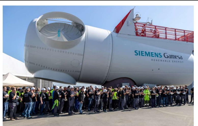
Figure 7-5. Scale of wind turbine components (11 MW nacelle shown here, 14 MW nacelles planned) (Source: Siemens Gamesa)
