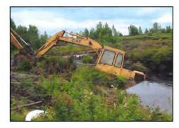
**B-522-2006 Deblois Worchester Peat Company** While cleaning out a channel in a pond designed to catch peat from the bog, an excavator slid off of the dike that it was traveling along and into the pond. The equipment's engine was underwater releasing oil to the pond's surface. Protective sorbent boom was placed across the water. The excavator was successfully removed from the pond a few days later.
