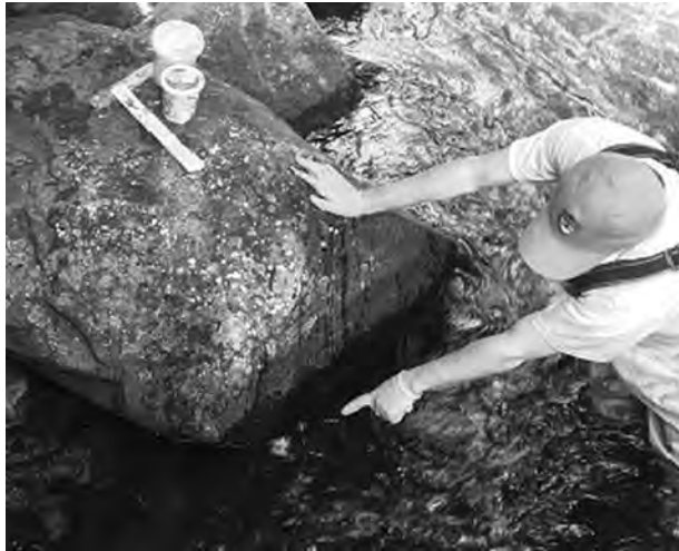
Figure 17. A temperature logger epoxied to the downstream side of a large boulder. MDIFW contractor Chris Introne is pointing to where it is attached.
