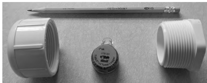
Figure 15. A Typical temperature logger (middle) and housing, using a pencil for scale.
