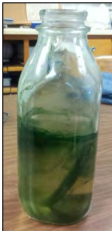
Figure 4. An advertised 100% biodegradable Berkley® Gulp!® sinking minnow SPL was placed in Kennebec River water to evaluate degradation over time (Left). The SPL was checked at 1 week, 1 month, and 8 month intervals. No signs of degradation were documented during this cursory study (Right).
