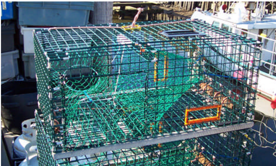
Photo 2. A regulation lobster trap, with the funnelled opening on the left hand side of the trap, in the middle can be seen the funnel that leads to the parlour. An orange plastic rectangular escape vent can also be seen on the bottom right side of the trap.
