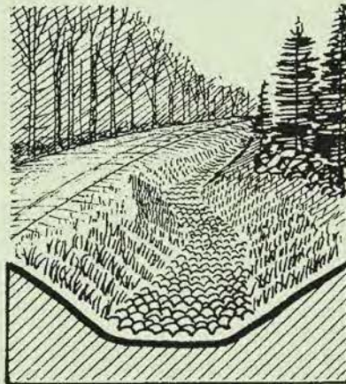
Grass and stone stabilized ditch
