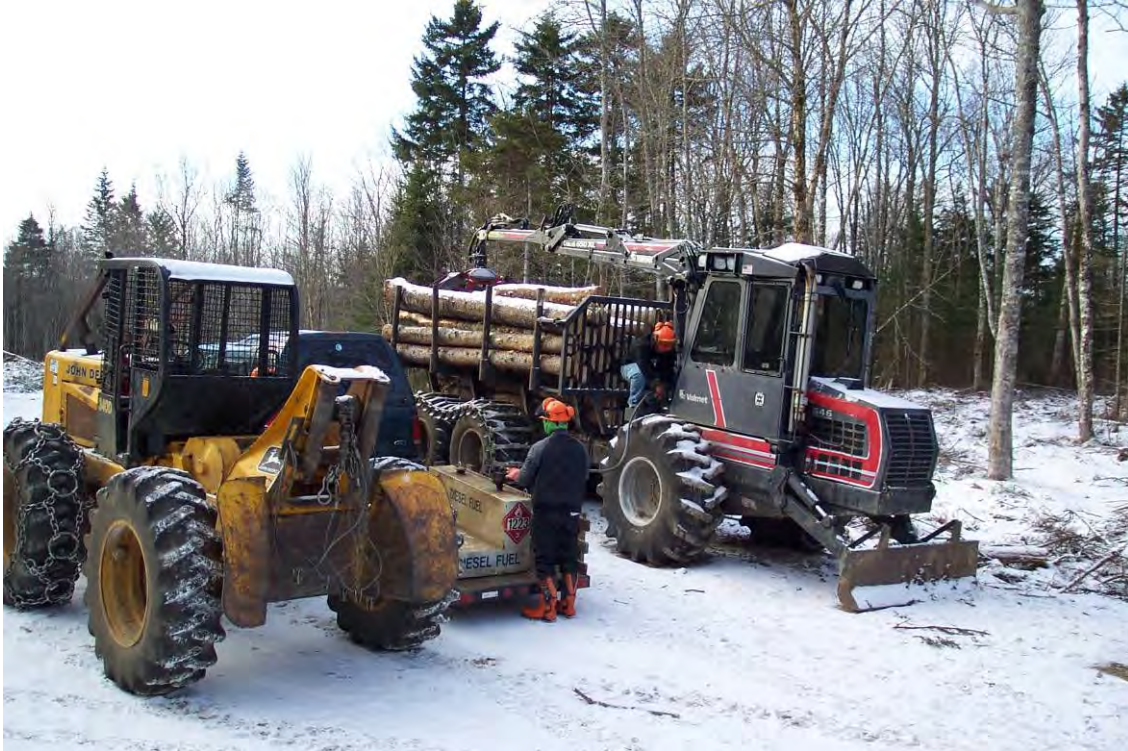
When used properly carried wood systems (e.g. the forwarder seen on the right) can result in less soil disturbance vs. dragged wood systems (e.g. the cable skidder seen on the left). Regardless of the type of system used, operator skill and training are critical to good results.
