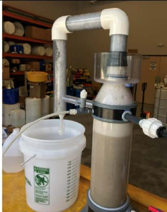
Figure 2. Bench foam fractionation unit used for testing
