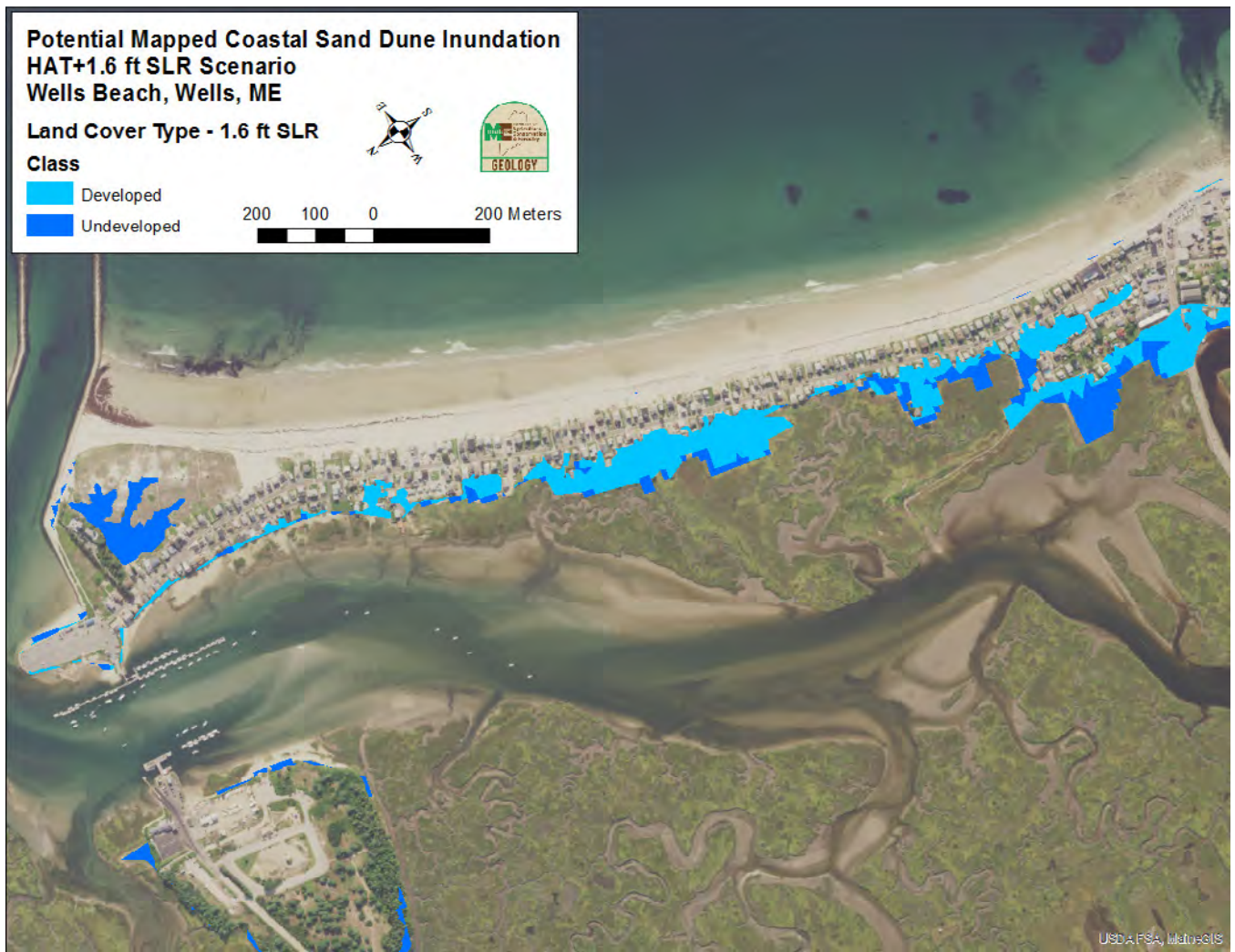
Appendix D, Image 1. Potential inundation of developed and undeveloped coastal sand dunes in Wells, ME after 1.6 ft of SLR.
