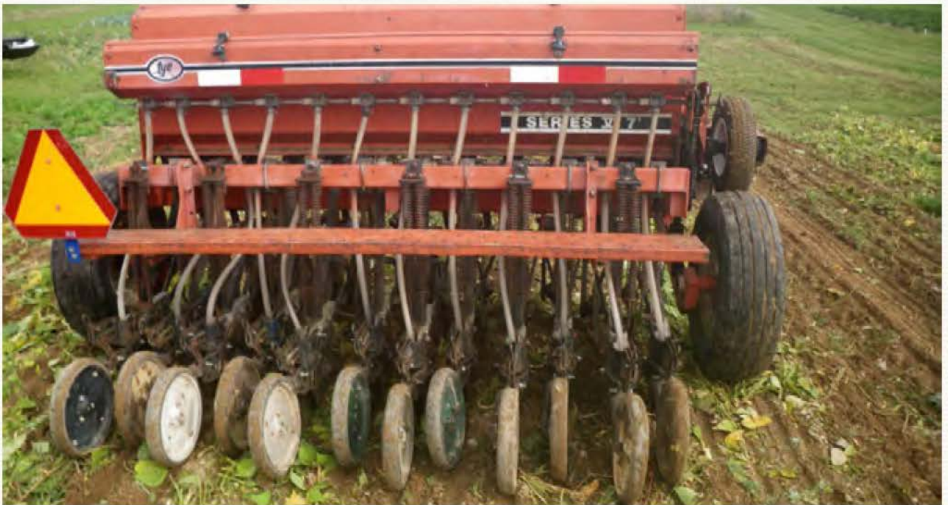
The District's no-till seeder, which they own and rent out to other farmers, which helps get seed in the ground while reducing runoff and erosion.
