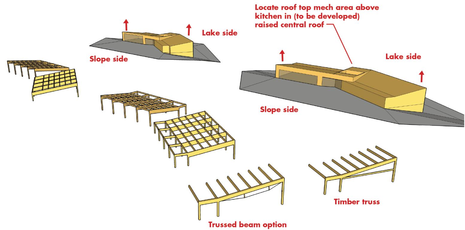
Lodge Roof - Mass Timber Structural Diagrams - NTS
