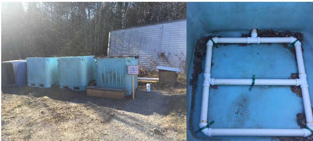
Figure 2. Aerated compost bin system located at Vinalhaven transfer station. Photos by Mark King.
