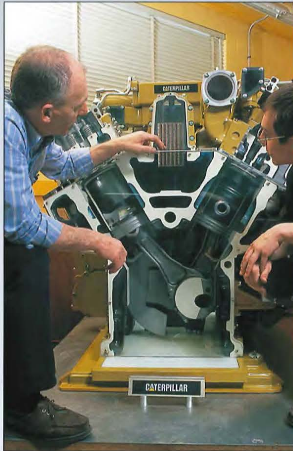
Our working cutaway diesel engine provides a glimpse of the machine's inner workings.
