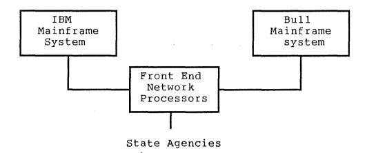
The network processing units route traffic from a particular customer to the appropriate mainframe system. Many Bureau customers communicate with the mainframe system over a network of data communications equipment which is provided and maintained by the Bureau. Some customers communicate directly with the mainframe system over the network; others prepare the data themselves and deliver it to Bureau of Data Processing for processing by the mainframe systems.
