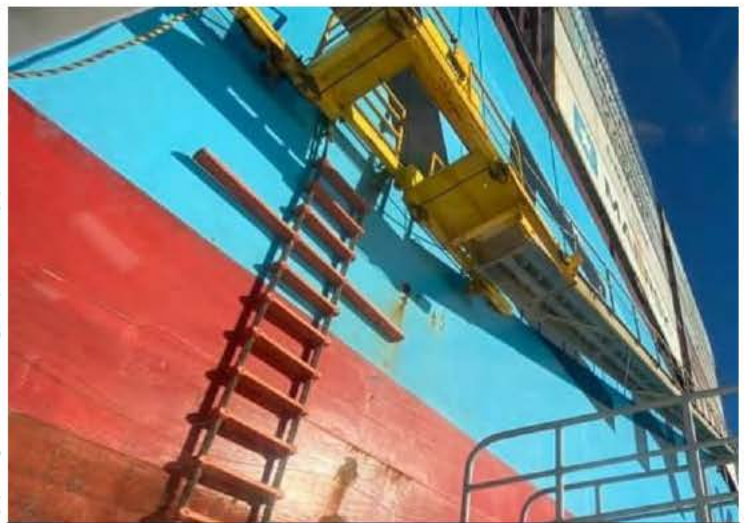
Example of trapdoor arrangement with ladder hanging from the bottom of the platform.
