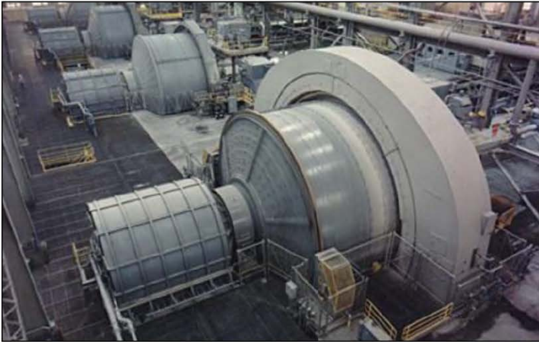
Rotating ball mill. Used for grinding ore to a fine particle size.
