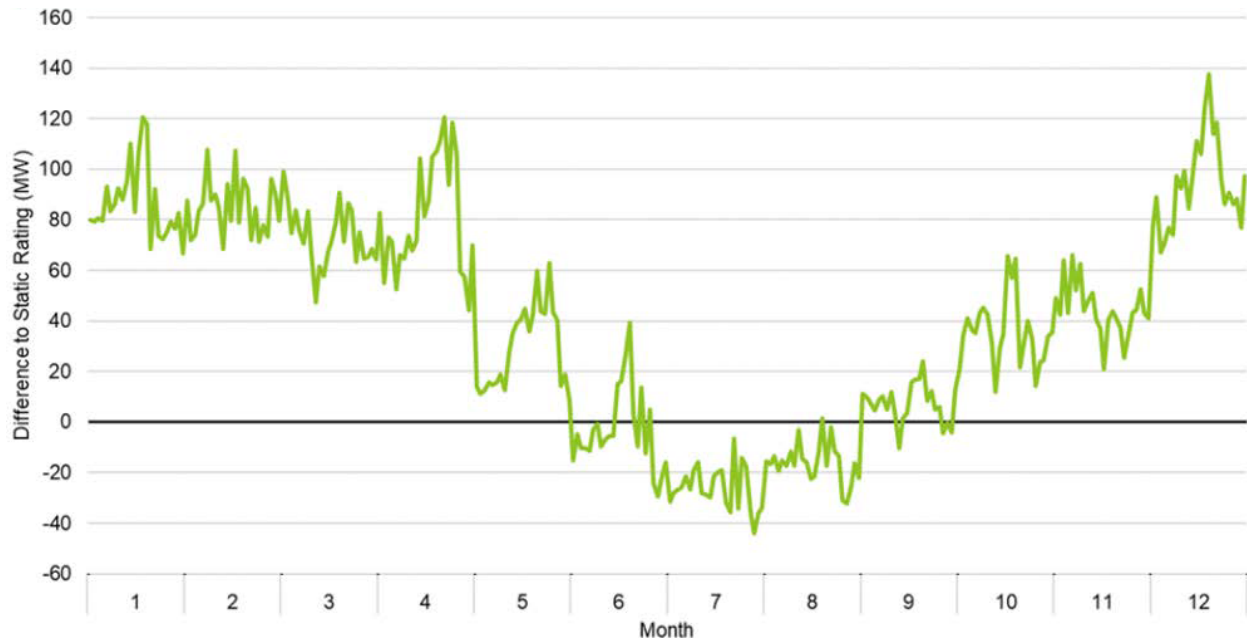
Figure 13: Differences between DLRs and Static Line Ratings, Canandaigua to Avoca Line
