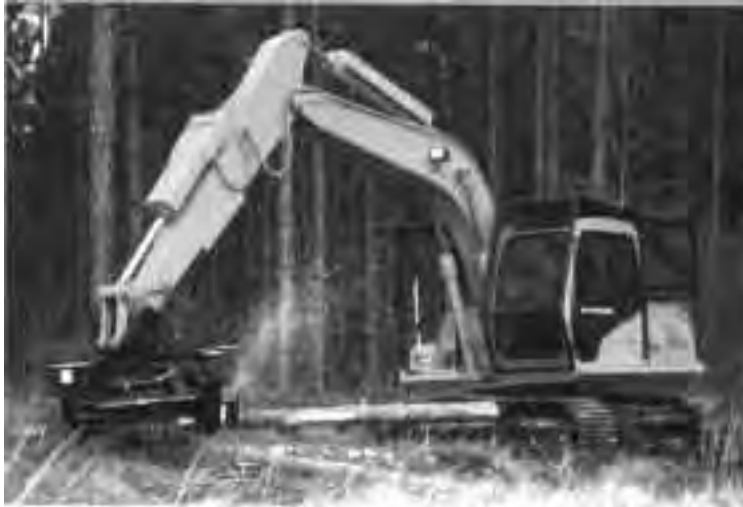
CTL "Processor". Hahn Machinery photo.
