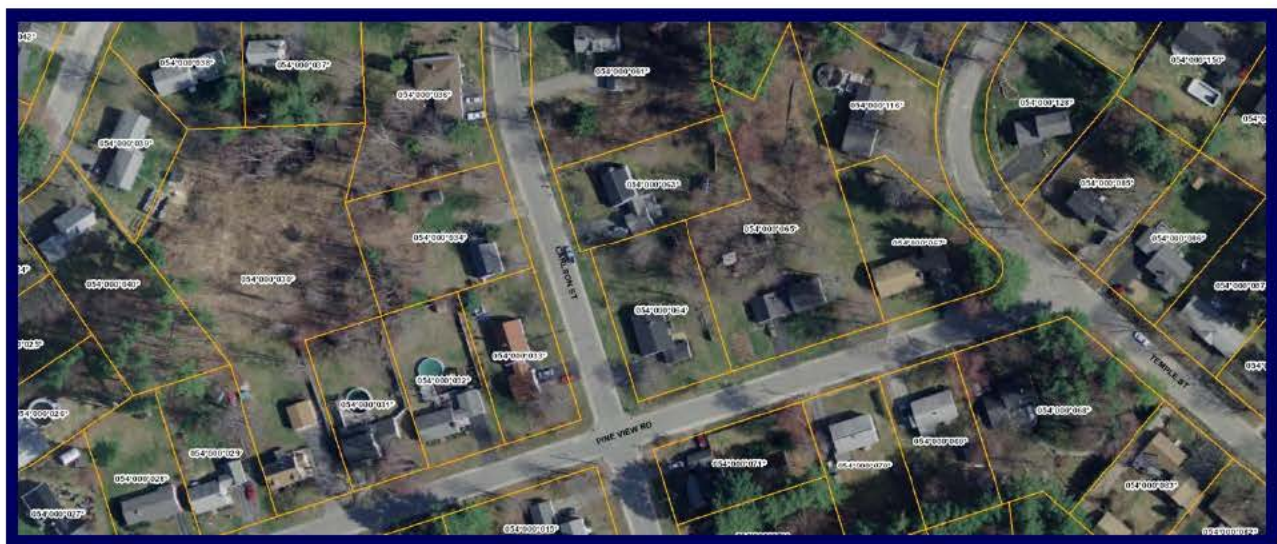
Figure 8. Parcel data with orthoimagery overlaid beneath it. An example of using multiple geospatial data layers.
