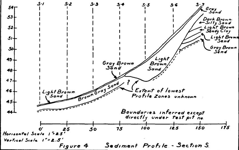
Figure 4 Sediment Profile - Section S.
