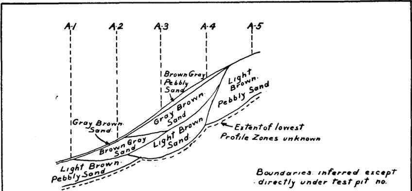
Figure 1 Sediment Profile Section A.
