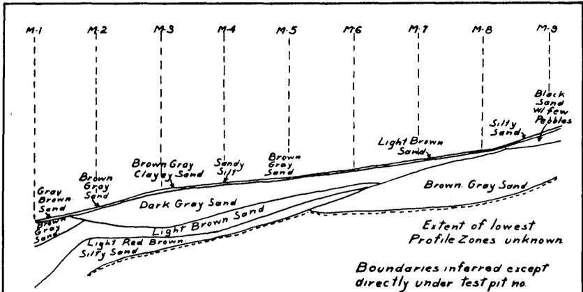
Figure 3. Sediment Profile, Section M
