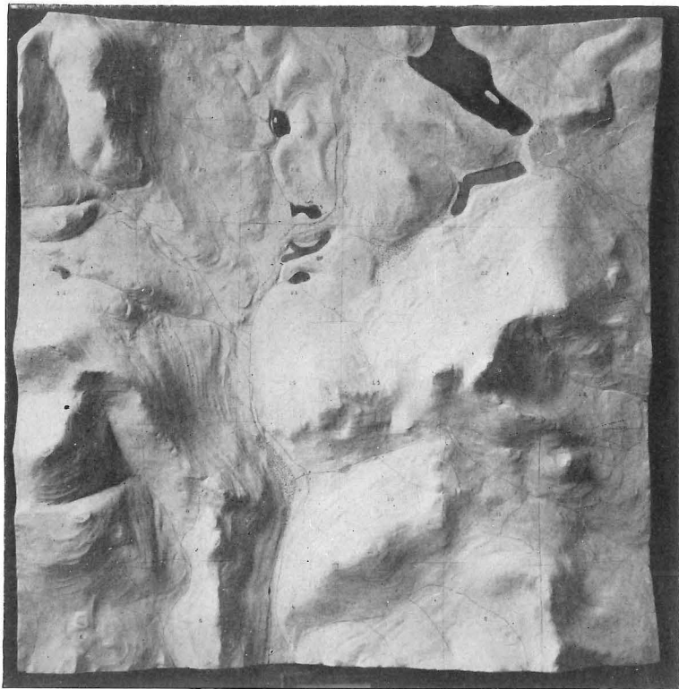
Topographical model of Township No. 3, R. 5, Franklin County, Maine, showing in addition to the waters, relief bogs, roads, trails, section lines, etc.
