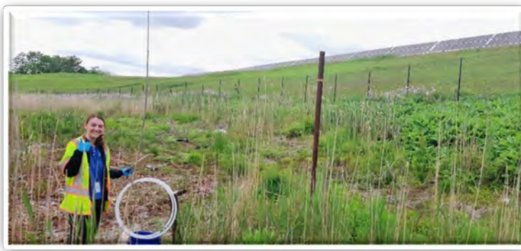
Developing a monitoring well at a landfill
