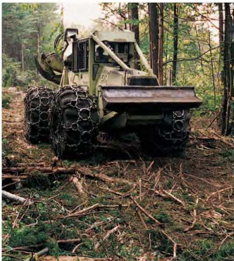
Brush on skid trails, as well as frozen ground, helps minimize soil disturbance and rutting.
