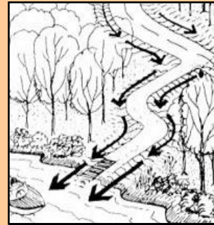
Improperly constructed and/or maintained shore-side roads can result in sedimentation to lakes and ponds.
