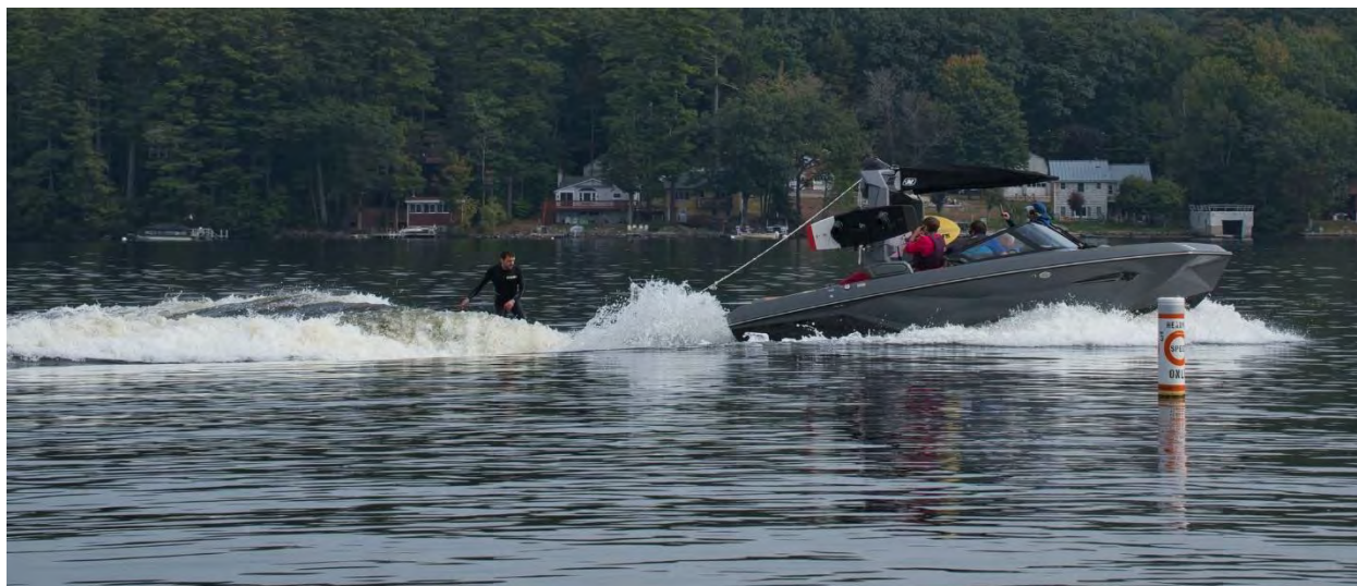
2023 Nautique G21 being utilized in “wakesurf mode”. Wakesurf mode consists of full ballast, speed set for 11.6 MPH, surf system deployed. Surfer has successfully dropped the rope and is not attached to the boat.
